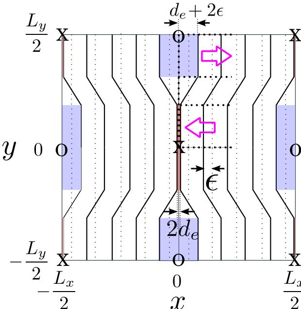
...  $\left( \text{Contours of } \psi_e \text{ are deformed into a "Y-shape".} \right)$
