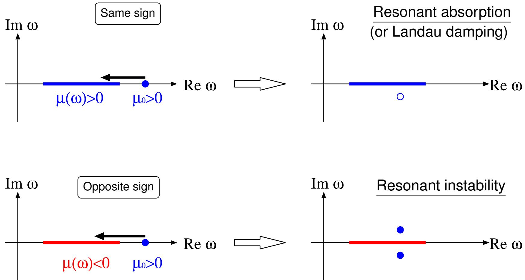
By using the averaged Lagrangian method (assuming  $\text{Re } \omega \gg 0$ ), adiabatic invariance of the total wave action  $\mu_0 + \int \mu(\omega) d\omega$  holds. [Hirota & Tokuda, PoP 17, 082109 (2010)]
