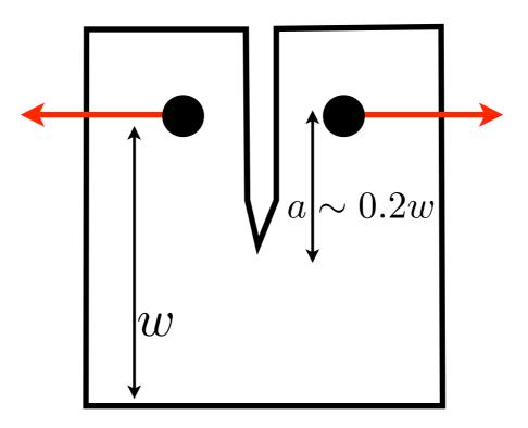
fracture in thin sheets :: always bending
