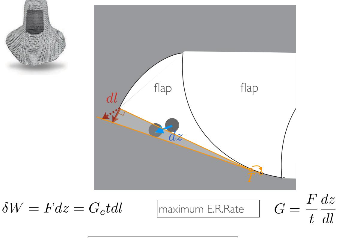
minimum advance dl of crack for fixed object step dz
