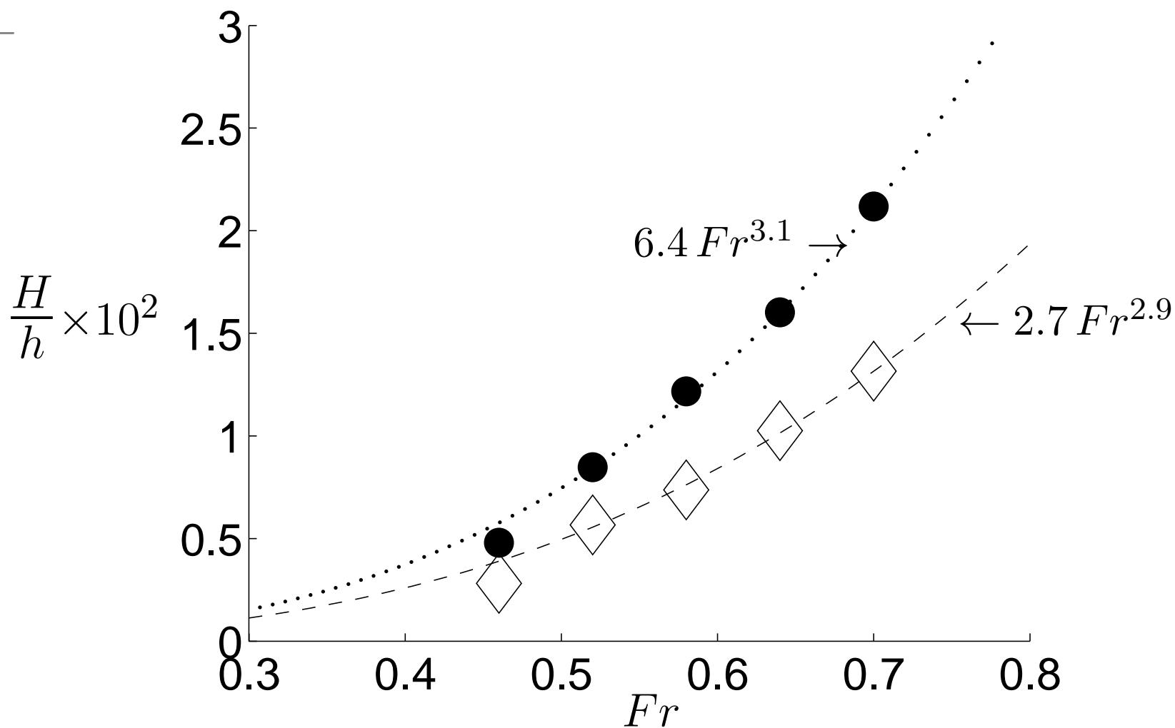
Max. wave height at channel wall (●) and ahead of ship (◇).
