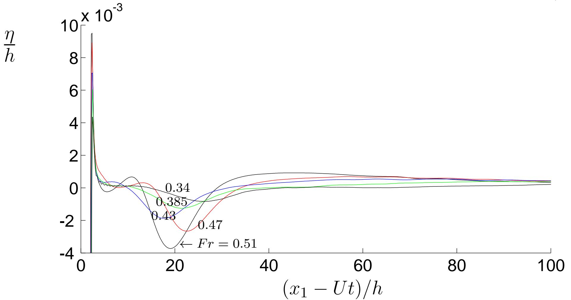
Ship moving from depth  $h - \frac{1}{2}\Delta h$  to depth  $h + \frac{1}{2}\Delta h$ .
