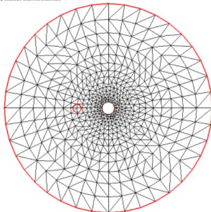
**Figure:** Test 1 – The initial geometrical configuration, the initial triangulation and the target  $D$ . Number of triangles: 992; number of vertices: 526.
