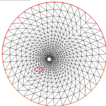
**Figure:** Test 2 – The initial geometrical configuration, the initial triangulation and the target  $D$ . Number of triangles: 1206; number of vertices: 633.
