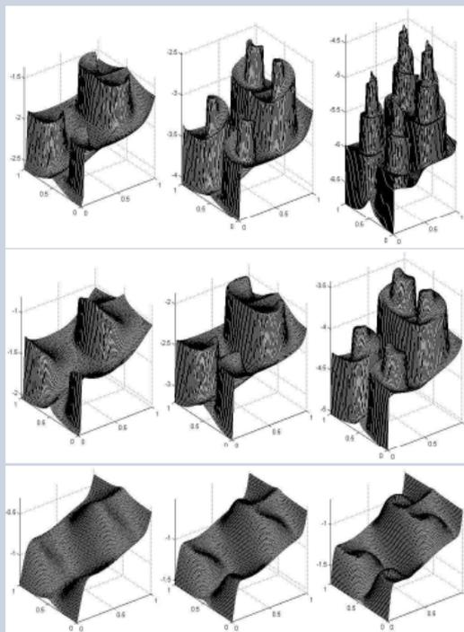
Graphs of  $G(x, 1)$  for inviscid (1st row in  $A = 4, 8, 16$ ), curvature, viscous G-equation with  $s_L = 1$ ,  $P = e_1$ ,  $d = 0.1$ .
