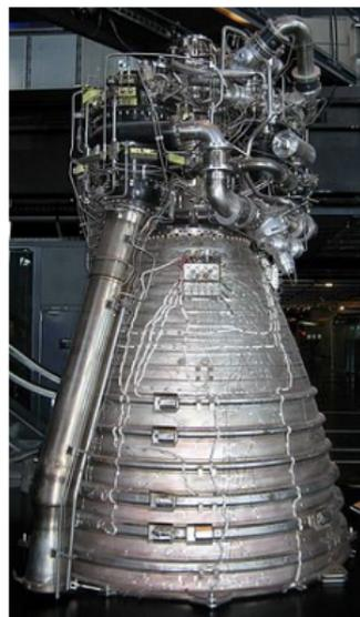
Figure: Vulcain engine for Ariane 5; CC-by-sa 3.0, Pline, Wikimedia Commons
