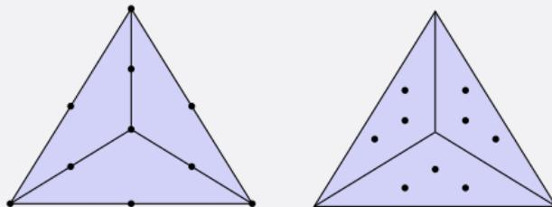
Quadratic Lagrange velocity element (left) and discontinuous linear pressure space (right) form a stable finite element pair on Alfeld splits.
