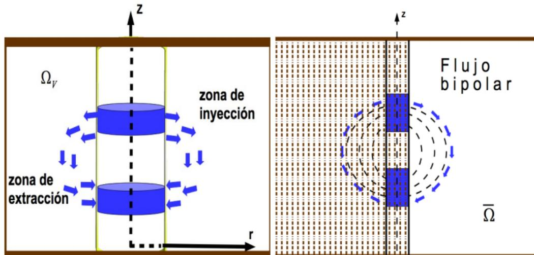
Two screening sections are drilled by a well seal. A tracer pulse is introduced into the fluid by the injection screening section, and is extracted through the other zone.
