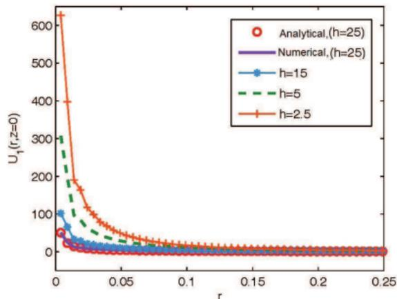
Pressure gradient and radial velocity near the wellbore increase as the screening zone thickness  $h$  decreases
