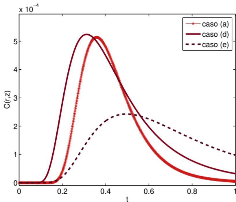
Concentration profiles at the midpoint of the extracted zone that show the sensitivity to thickness of the layers.
