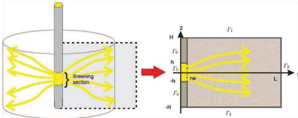
Our goal is to analyze the tracer behavior in partially penetrating injection wells when the vertical component of velocity is taken into account
