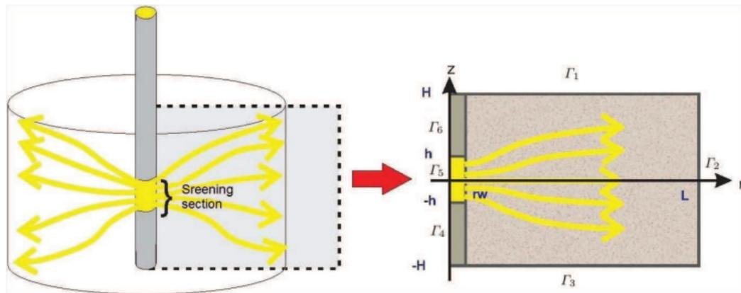
$\bar{\Omega} = [r_w, L] \times [-H, H]$ , cylindrical coordinates with fixed  $\theta$
