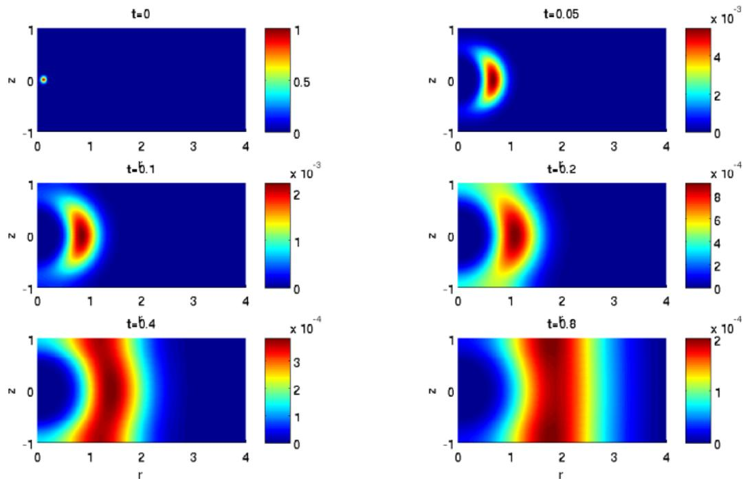
Pulse dynamics for  $D = 0.05$  and purely radial velocity (fully penetrating well)
