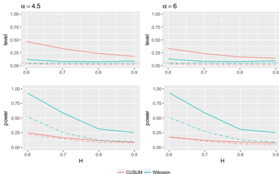
Rejection rates of the CUSUM and Wilcoxon tests for LMSV time series of length  $n = 500$  with Hurst parameter  $H$ , tail index  $\alpha$  and a shift in the variance in  $\tau = 0.25$  with height  $h = 0.5$ . The calculations are based on 5000 simulation runs.
