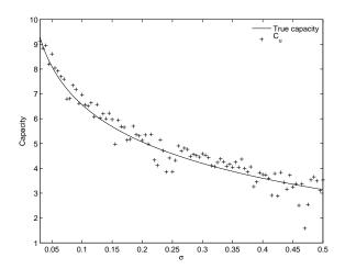
$C_u$  for L=50 observations, n=4 receive antennas, m=4 transmit antennas, with varying values of  $\sigma$ . With phase drift and phase off-set. The rank of  $\mathbf{H}$  was 4.
