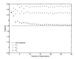
Comparison of the classical capacity estimators for various number of observations.  $\sigma^2=0.1,\ n=10$  receive antennas, m=10 transmit antennas. The rank of **H** was 3.
