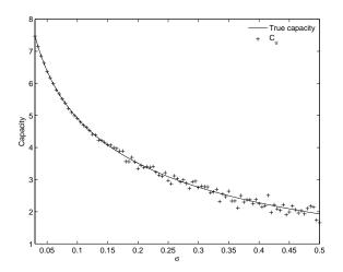
$C_u$  for L=10 observations, n=4 receive antennas, m=4 transmit antennas, with varying values of  $\sigma$ . With phase drift and phase off-set. The rank of  $\mathbf{H}$  was 3.
