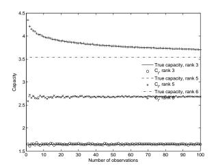
$C_f$  for various number of observations. No phase off-set/phase drift.  $\sigma^2=0.1$ , n=10 receive antennas, m=10 transmit antennas. The rank of **H** was 3, 5 and 6.
