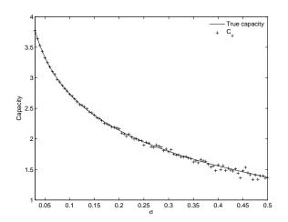
$C_u$  for L=1 observation, n=10 receive antennas, m=10 transmit antennas, with varying values of  $\sigma$ . With phase drift and phase off-set. The rank of  ${\bf H}$  was 3.
