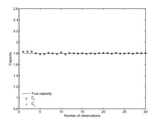
Comparison of  $C_f$  and  $C_u$  for various number of observations.  $\sigma^2 = 0.1$ , n = 10 receive antennas, m = 10 transmit antennas. The rank of **H** was 3.
