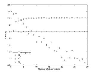
Comparison of capacity estimators which worked when no phase off-set/drift was present, for increasing number of observations. With phase drift and phase off-set.  $\sigma^2 = 0.1$ , n = 10 receive antennas, m = 10 transmit antennas. The rank of **H** was 3.
