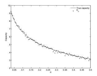
$C_u$  for L=1600 observations, n=4 receive antennas, m=4 transmit antennas, with varying values of  $\sigma$ . With phase drift and phase off-set. The rank of  $\mathbf{H}$  was 4.
