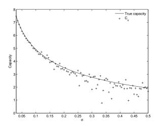
$C_u$  for L=1 observation, n=4 receive antennas, m=4 transmit antennas, with varying values of  $\sigma$ . With phase drift and phase off-set. The rank of **H** was 3.
