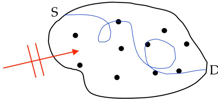
Fix the source and detector and measure the transmitted intensity as the wavevector of the acoustic wave is varied
