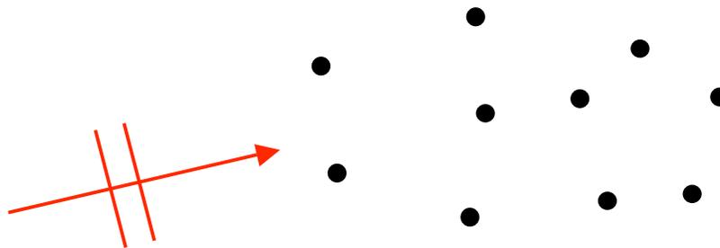
Consider a fluid suspension of scattering particles on which an acoustic wave is incident. The acoustic wave leads to **spatial modulation** of the number density of scatterers and the speed of light in the medium. If the amplitude of the pressure wave is sufficiently small, each particle will oscillate independently about its local equilibrium position. The equation of motion of a particle with velocity  $\mathbf{u}$  is of the form
