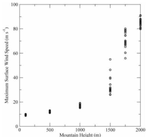
FIG. 5. Maximum leeside wind speed ( $\text{m s}^{-1}$ ) at the lowest model level (100 m) for each ensemble member as a function of the mountain height (m) at the 4-h simulation time.
