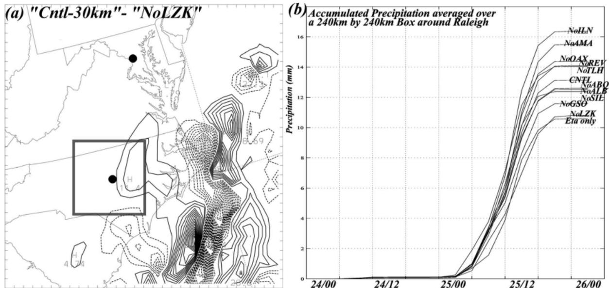
FIG. 15. (a) The 36-h accumulated precipitation difference (every 4 mm) between Cntl-30km and NoLZK. (b) Time evolution of the accumulated precipitation (mm) averaged over a 240-km  $\times$  240 km box around Raleigh, NC, from each individual sounding experiment, Cntl-30km and EtaOnly. The location of the box is shown in (a).
