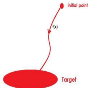
In  $\mathbb{R}^N$ , finding the **weighted distance** from a given target set is equivalent to solve the Eikonal equation  $|Du(x)| = f(x)$  with  $u = 0$  on the target.
