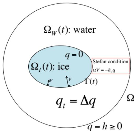
Figure: melting ice  $\Omega_I(t)$
