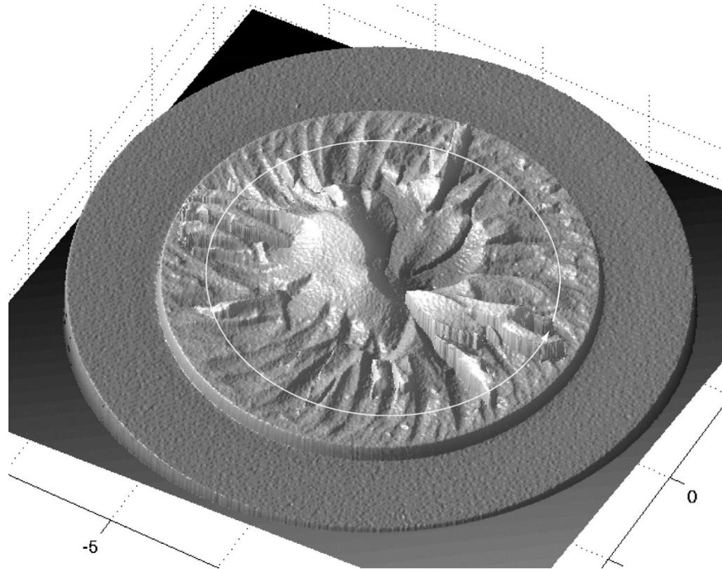
Typical spacing of facets along initial crack line is .07 mm
