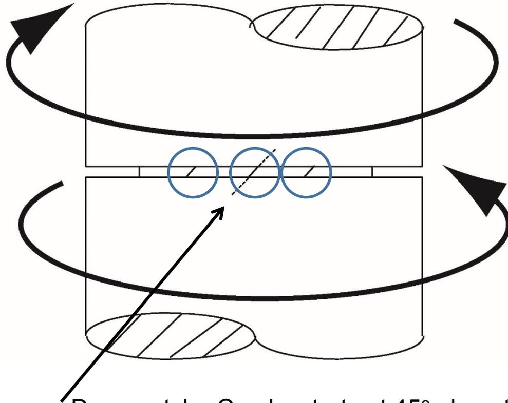
Deep notch. Cracks starts at 45° along the crack front. If these grow in vertical direction they run into region of larger net diameter and lower stress
