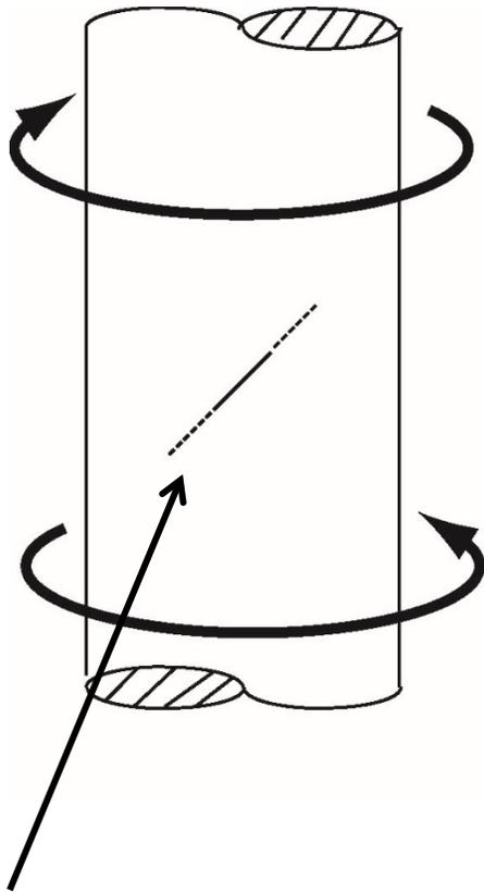
No or shallow notch, crack starts at 45° grows in vertical direction into uniform stress field. Spiral crack forms
