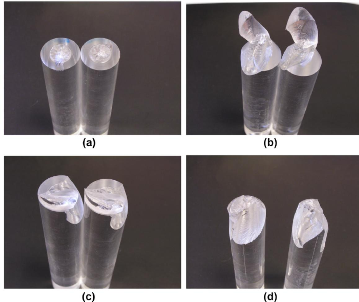
Fig. 6. Failure modes in some specimens with  $d = 5$  mm: U-notch,  $R = 0.5$  mm (a), V-notch,  $R = 2$  mm, (b). Failure modes in some specimens with  $d = 2$  mm: U-notch,  $R = 0.5$  (c), V-notch,  $R = 1$  mm (d).
