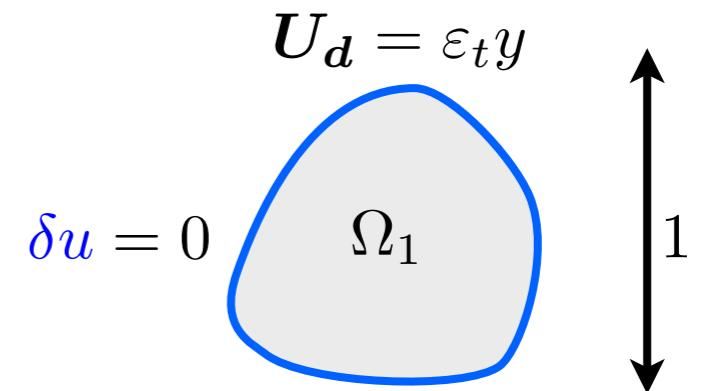
$$R_L(\delta u, \delta \alpha) = \frac{\int_{\Omega_1} A(\alpha_t) (\varepsilon(\delta u) - e_t \delta \alpha) \cdot (\varepsilon(\delta u) - e_t \delta \alpha) dy + w_1 \frac{\ell^2}{L^2} \int_{\Omega_1} \nabla \delta \alpha \cdot \nabla \delta \alpha dy}{\left( \frac{1}{2} S''(\alpha_t) \sigma_t \cdot \sigma_t - w''(\alpha_t) \right) \int_{\Omega_1} (\delta \alpha)^2 dy}$$
