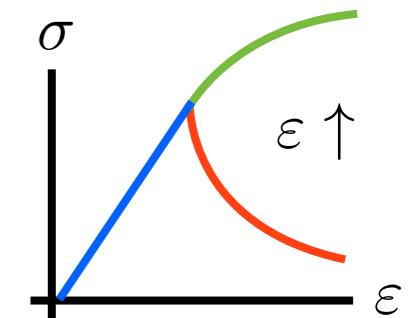
**Stress-hardening:** elastic space is increasing in stress space
