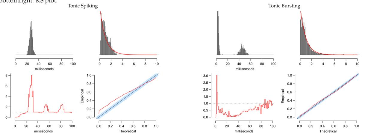
For Tonic Spiking the ISI histogram shows regular spiking patterns at  $\approx 27$ ms. The filter below show peaks at multiples of the ISI mean,  $q \cdot 27$ ms, for  $q = 1, 2, 3$ , respectively. The rescaled spike times and the KS plot both show, that the model tends to overestimate smaller ISIs and slightly underestimate longer ISIs.
