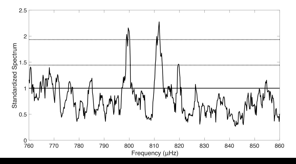
Periodogram of data using high pass filtering, pre-whitening and post-whitening
