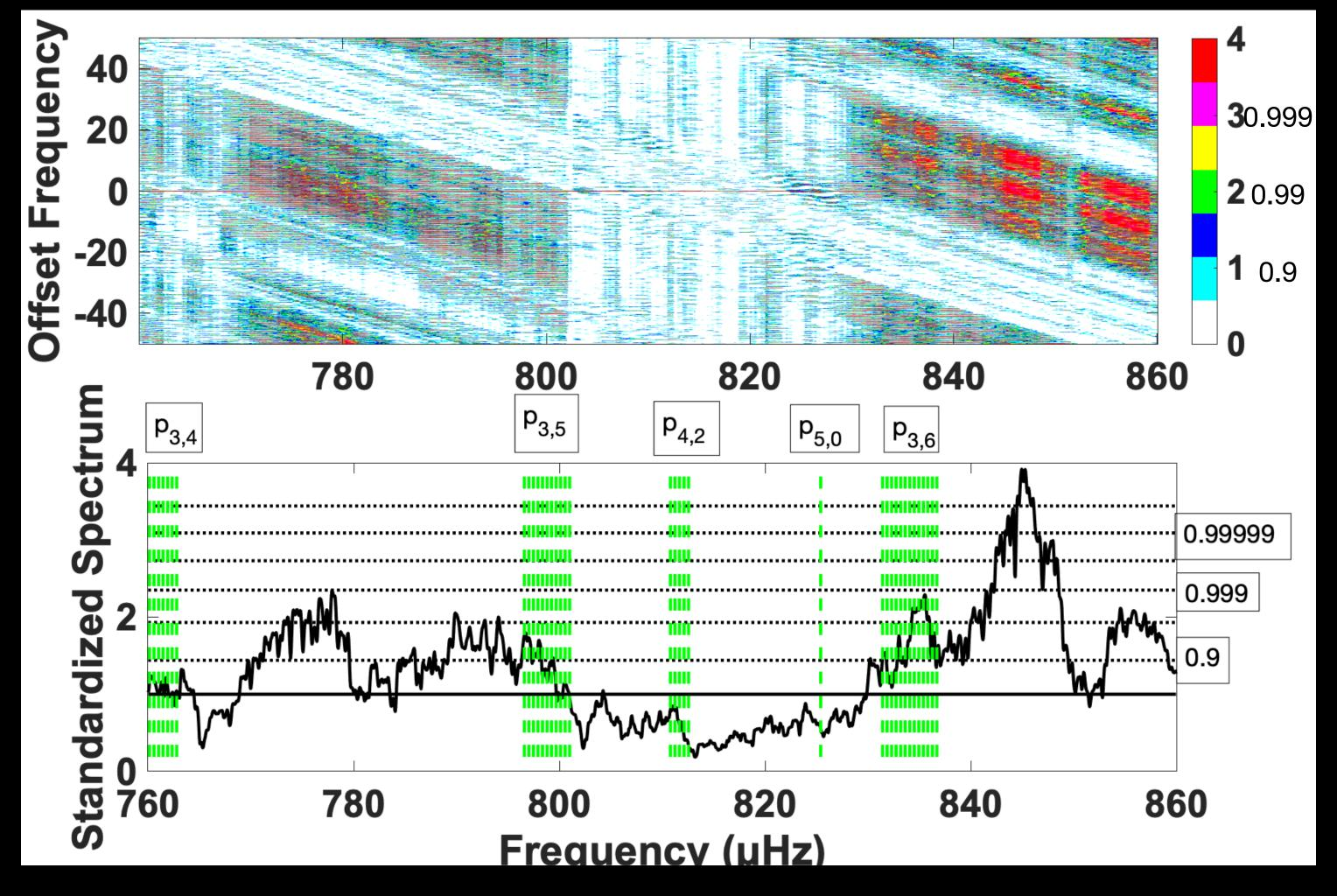
Trapezoidal block: if  $f_1$  is coherent with  $f_2 > f_1$ , then the coherence will be high at positive offset frequency  $f_2 - f_1$  and also at negative offset frequency  $f_1 - f_2$  at frequency  $f_2$
