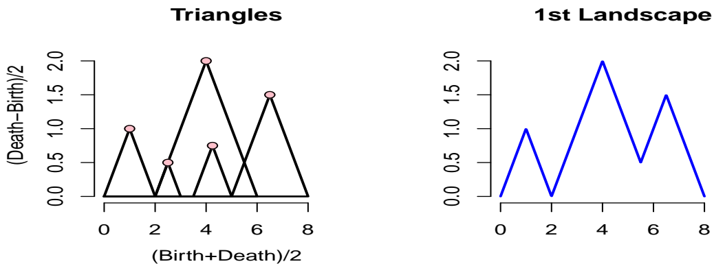
Figure 1: Left: we use the rotated axes to represent a persistence diagram D . A feature (b, d) \in D is represented by the point (\frac{b+d}{2}, \frac{d-b}{2}) (pink). Right: the blue curve is the landscape \lambda(1, \cdot) .
