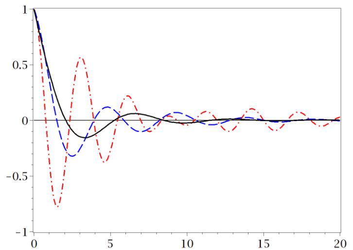
*Plot of  $h(\Omega, r)$  in  $GF_1$  theory as functions of  $r$  for different values of  $\Omega / \mu$ : 0 (solidline) and 2 (dashedline).*
