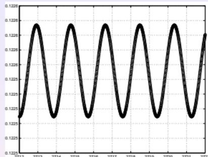
**Figure:** Driven Cavity for  $Re = 10000$  : Max streamfunction. Computations are done with  $N = 65$ , with  $\Delta t = 1/90$ .
