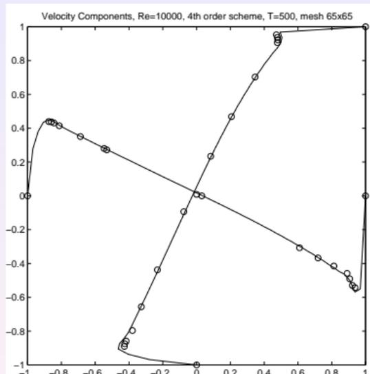
**Figure:** Velocity components for the driven cavity problem. Left:  $Re = 7500$ , fourth-order scheme with  $N = 65$  (solid line), Ghia-Ghia-Shin. with  $N = 257$  (circles). Right:  $Re = 10000$  fourth-order scheme with  $N = 65$  (solid line), Ghia-Ghia-Shin with  $N = 257$  (circles).
