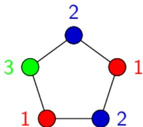
$$\begin{array}{c} \textcircled{c} \\ x \end{array} \text{---} \begin{array}{c} \textcircled{d} \\ y \end{array} \Rightarrow c \neq d$$
