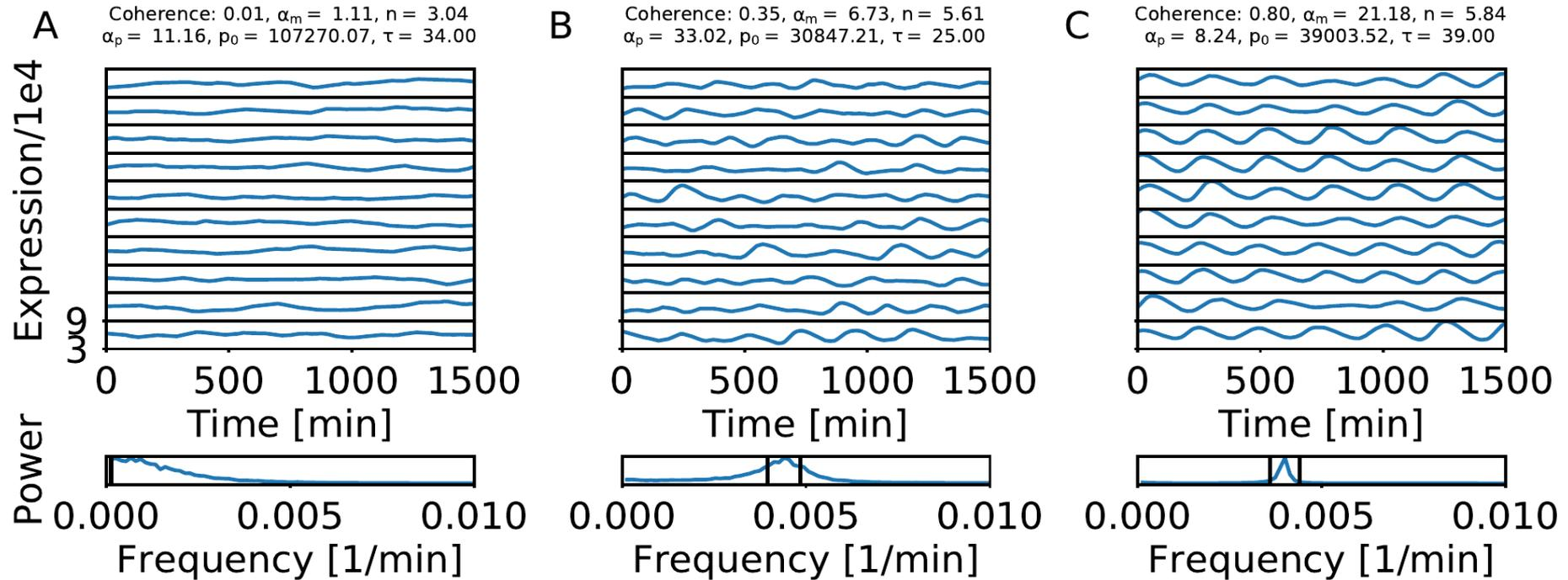
The model correctly predicts the period and amplitude of the oscillations
