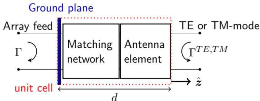
The reflection coefficient  $\Gamma^{TE}$  is bounded and passive, with help of a Blaschke-product  $B$  we find that  $-j \ln(\Gamma^{TE} B)$  is a Herglotz-function, and sum-rules apply.
