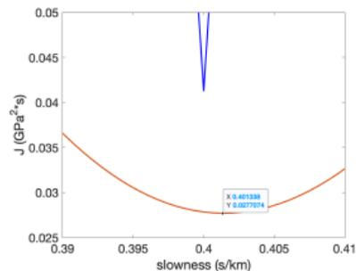
Left: data with noise. Middle: reduced FWI and ESI objective functions versus slowness. Right: Zoom in of middle figure.
