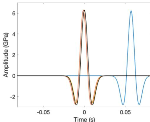
Left: Estimated wavelets. Right: truncated estimated wavelets. Blue curve is the initial wavelet. Red curve is the estimated wavelet after the first update of  $m$ . Yellow is the estimated wavelet after the final  $m$  update. Black curve is the target.
