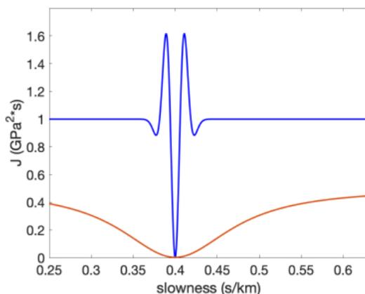
The FWI (blue curve) and ESI (red curve) objective functions versus slowness for data from a 40 Hz Ricker source.
