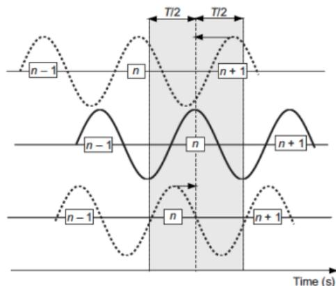
Schematic of cycle-skipping artifacts in FWI. Solid black line is seismogram of period  $T$ . Upper dashed line is seismogram with a time delay greater than  $T/2$ . Bottom example, has time delay less than  $T/2$ .<sup>1</sup>
