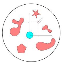
E.g., impossible for this differential drive robot to stably aim within  $\pm 179$  degrees of the origin while "strictly" avoiding obstacles.
